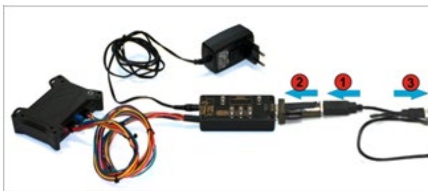
Figure 6: Connecting the converter with the USB cable
